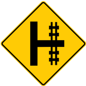
Railway crossing on side road ahead — be prepared to stop
